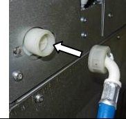
OVEN WATER CONNECTION AT REAR
