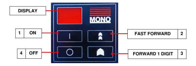
**2.0** Press the panel (2) to move the display to the required number.
