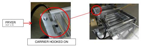
Screws at bottom of carrier have been tightened. (Unlikely but should be loose to allow up/down movement).
