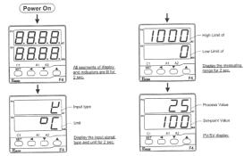
Figure 4. Powering up procedure
