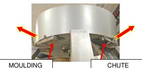
MOVE DUSTER CONTROL PLATES TO CONTROL THE FLOUR IN THE AREA REQUIRED. THE MORE HOLES SHOWING, THE MORE FLOUR FLOWS
