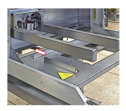
This allows different width trays to be accommodated. To adjust the position of the back guide, remove the table and turn it over. Loosen the thumb nuts and slide the sheet across to the desired position. Tighten the nuts and replace the table.
