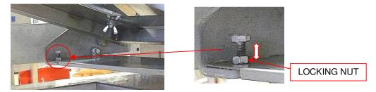
Lift the front edge of the table and, with a suitable spanner, release the locking nut. Screw the adjuster bolt up or down and then lock it in position with the locking nut.
