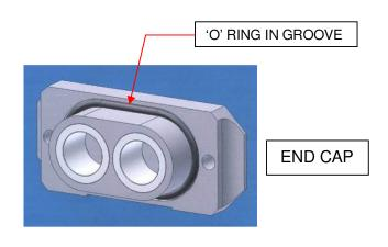
4. To fully dismantle pump assembly components for cleaning, remove remainder of pump assembly from the machine and remove remaining end-cap.
