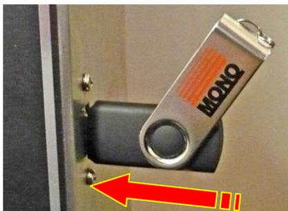
Insert the USB memory stick into the socket on the side of the oven panel. (Rubber plug may have to be removed first).
