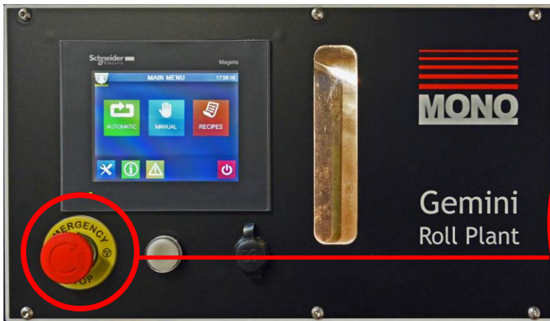
Touch Control Panel
