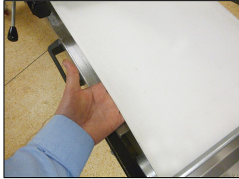
Lower Belt Tensioning
