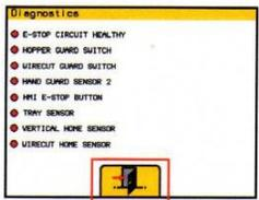
Test that **ALL** inputs are working correctly using the diagnostics page.
