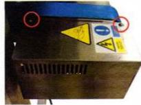
To access the tray motor remove the cover plate. There are 2 screws on the top and 2 screws on the bottom
