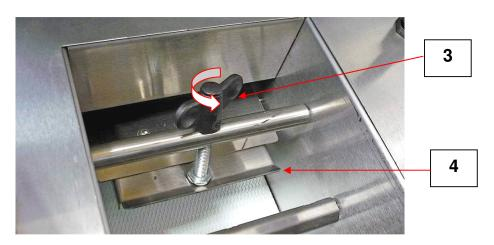
4 Remove cover on top behind hopper. Loosen wing bolt (3) and lift out rear scraper (4). Wipe clean and refit.
