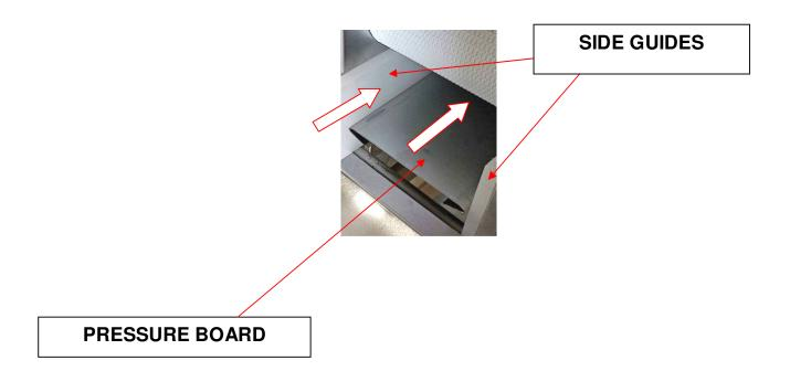
To reduce the width of the dough path for finger rolls etc. the side guides and pressure board have to be changed.
