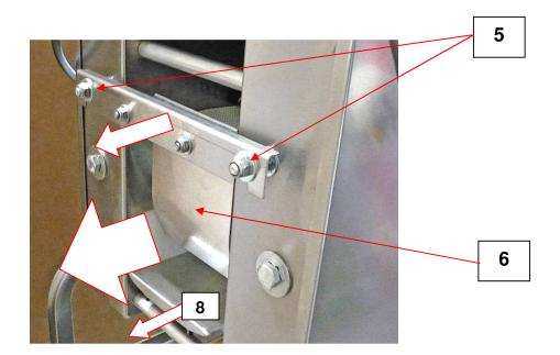
6 Remove side cheeks (7) by sliding out of machine to the rear. Wipe clean.
