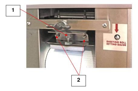
3 Turn down knurled bolt (1) and withdraw front scraper from retaining hooks (2). Wipe clean and replace.
