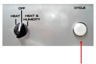
Next to the control switch is an **indicator light** to show when the cabinet is heating. To help maintain the humidity and temperature levels, try to keep the door closed when this light is illuminated.
