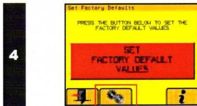
Press the **SET FACTORY DEFAULTS BUTTON**. Then press The **COGS** Button to enter the System Menu.
