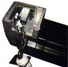
Slide the cable gland plate from the motor housing to gain access to the connectors.
