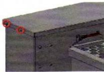
Remove the 4 screws securing the main enclosure lid (2 on each side) using 1 4mm allen key and 10mm spanner/socket to gain access to the electrical control panel. To remove the lid lift the lid at the front and slide to the rear then lift to remove.
