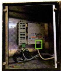
Connect the HMI cable to the connector marked ETHERNET. Ensure that the cable is pushed in firmly, you should hear a "click".
