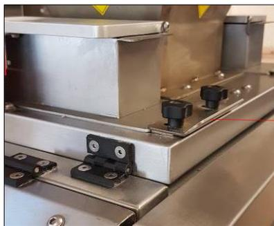
*Slide the Retaining Plate to the Unlocked Position on Each Sides of the Flour Duster*
