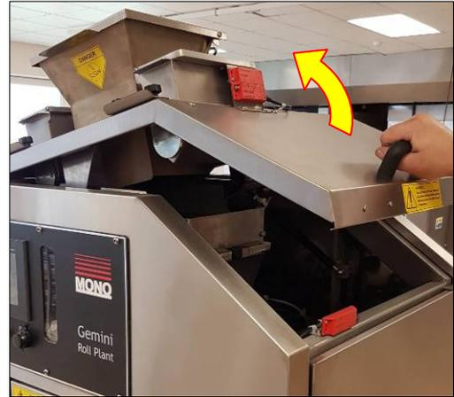
*Lift the Outer Access Door Upwards*
