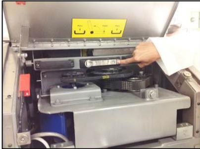
*Press the Button to Release the Handle*
