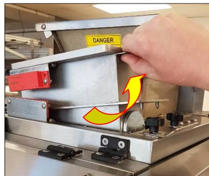
*Lift the Front of the Flour Duster Upwards to Remove and Insert the Cog-End First in Order to Replace*
