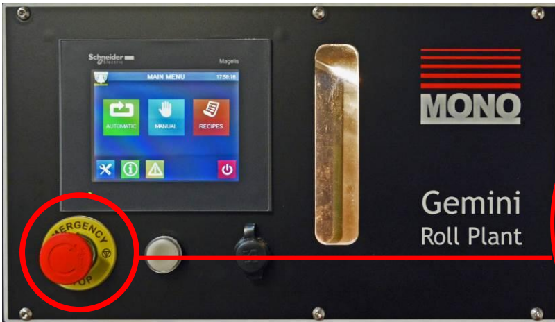
Touch Control Panel
