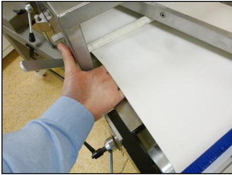
Upper Belt Tensioning
